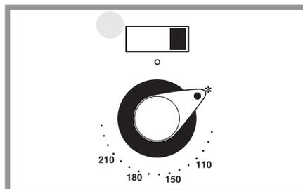
**5** \* The fan only setting. The fan circulates air inside the oven but the heating element is not turned on. This setting is useful for defrosting small quantities frozen foods.
