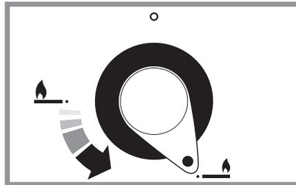
**2** Adjust the flame height to suit by turning the knob. On this cooker the low position is beyond high, **not** between high and off. The small flame marks the 'low position'. Turn the knob towards it after the contents of a pan have boiled.
