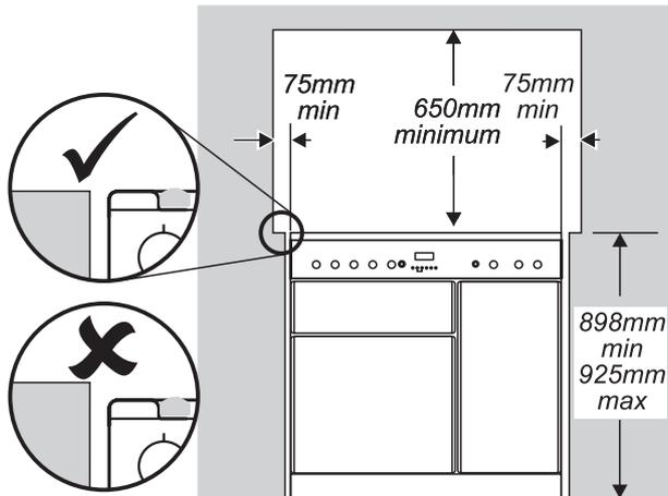
The hotplate surround should be level with, or above, any adjacent work surface. Above hotplate level a gap of 75mm should be left between each side of the cooker and any adjacent vertical surface.
