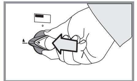
If when you let go of the control knob the burner goes out, the safety device has not held in. Turn off the grill and wait one minute then try again this time holding in the control knob for slightly longer.
