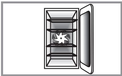
**4** The fan in the oven circulates hot air continuously, which means faster more even cooking.
