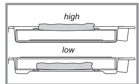
**7** The grill pan grid can be turned over to give two grilling positions.
