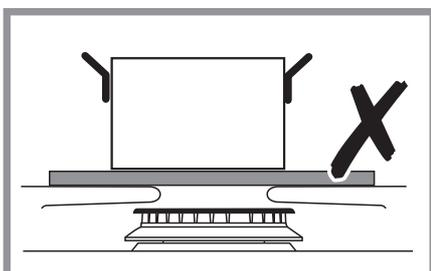
**4** Simmering aids, such as asbestos or mesh mats, are NOT recommended. They will reduce burner performance and could damage the pan supports.
