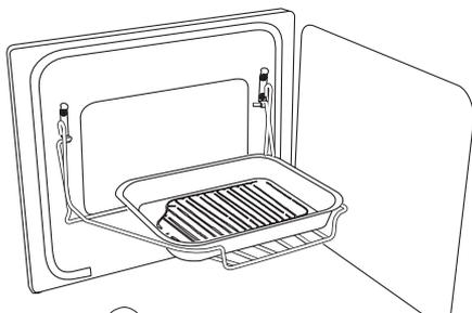
*The Handyrack fits to the left hand oven door only. Food cooking on it is easy to attend to, because it's accessible when the door is open. It can be fitted at two different heights. One of the oven shelves must be removed and the other positioned to suit.*
