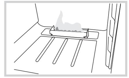
**3** The Main oven in your cooker use the our special 'Heatflow' system. Because the oven burner is not hidden under the oven base you will see the burner flames at the back of the oven - this is perfectly normal. Initially the gas will burn with a small flame but after approximately one minute the flame will become larger indicating that the oven is full on.
