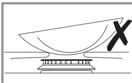
**5** Avoid using unstable and misshapen pans that may tilt easily and pans with a very small base diameter e.g. milk pans, single egg poachers. The minimum pan diameter recommended is 120mm (about 4<sup>3</sup>/<sub>4</sub>").
