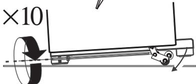
Make sure you lower BOTH REAR ROLLERS. There are two adjusting nuts, one for each roller, at both the front bottom corners of the cooker. Open the grill door and the Tall oven door. Grip under the fascia panel and lift the front of the cooker.
