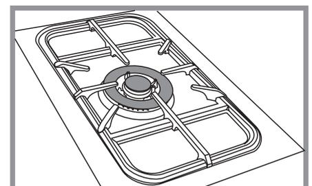
**6** The Wok burner is designed to provide even heat over a large area. It is ideal for large pans and stir frying. For heating smaller pans the smaller burners may be more efficient.
