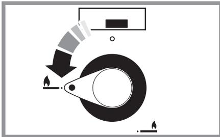
**1** The drawing by each knob indicates which burner that knob controls. Push in and turn a knob to the large flame symbol (🔥) and press the igniter button or light with a match.
