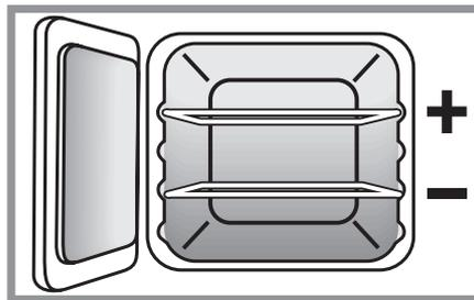
**5** Dishes placed above the central position will be cooked at approx. one gas Mark higher, dishes cooked below approx. one gas Mark lower. You can therefore cook dishes requiring different gas Marks at the same time.
