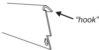
When refitting make sure that the trim is in the middle of the front of the oven burner bracket.
