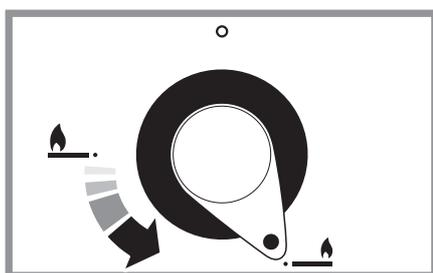
**5** The low position, marked with the small flame symbol, is beyond high, not between high and off.
