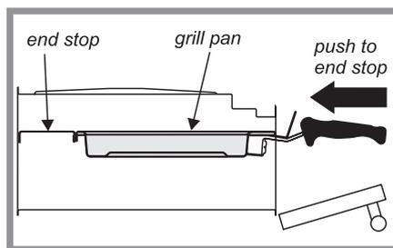
**6** For best results preheat for 2 minutes with the grill pan in position. After placing your food on the grill pan grid, slide the grill pan onto the side supports just below the burners. Adjust the flame height to suit by turning the knob.
