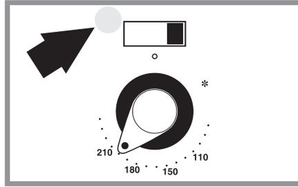
**2** The oven indicator light will glow until the oven has reached the temperature you selected. It will then cycle on and off during cooking.
