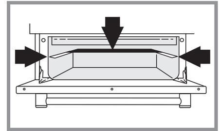
**3** After placing your food on the grill tray pan, slide the grill pan onto the side supports just below the burners. Make sure it is pushed right in and touches the back stop.
