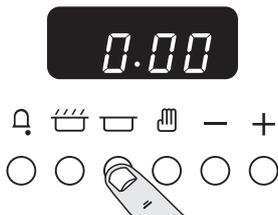
Press and hold as above. At the same time press (-) or (+) until your required 'Stop Time' shows. AUTO will show in the display. When your cooking is finished the beeper sounds. **TURN THE OVEN KNOB TO 0 FIRST**, then press once to stop the beep, press again to return to manual cooking.
