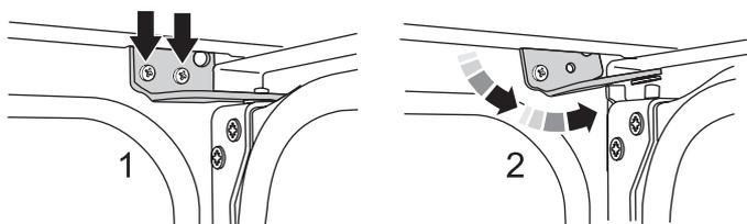
Support the weight of the door and remove the screw nearest the hinge pin. Swing the hinge up and away from the hinge pin on the door.
