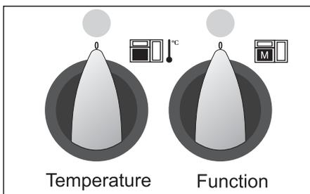
The Multi-function oven has two controls, a function selector and a temperature setting knob.
