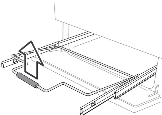
For safety, push the side rails back into the grill chamber.
