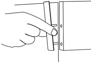
Pull off the push fit control panel end caps at each end and remove the end fixing screws under the end cap.
