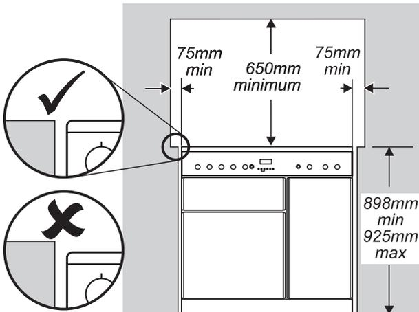
The hot surround should be level with, or above, any adjacent work surface. Above hotplate level a gap of 75mm should be left between each side of the cooker and any adjacent vertical surface.
