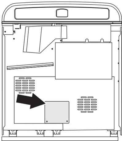
Connect the mains cable to the correct terminals for your electrical supply type. Please note the maximum cable size is 10mm<sup>2</sup> for the 3-pronged links.
