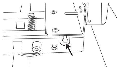
Make 10 complete (360°) turns clockwise. (This means turning and removing the levelling tool 20 times).
