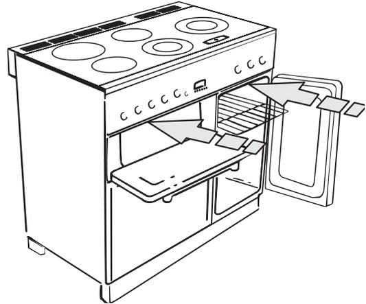
Open the grill door and right hand oven door so that you can get a good grip on the bottom of the fascia panel as you move the oven.
