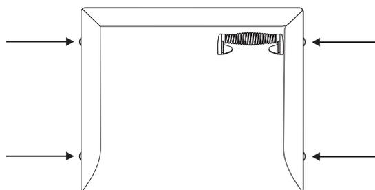
Remove outer door panel. Fit door handle to new panel. Fit the plastic blanking plugs to the fixing holes.
