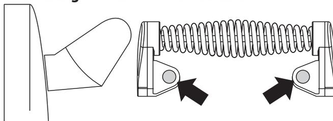
Remove the two plastic blanking plugs from the door handles. Remove the 4mm Hex headed screws holding the handle to the door with the hexagon key tool. Remove two screws from top edge and two from bottom edge of the door.
