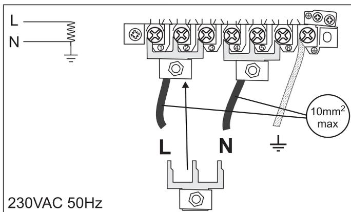
**Check that the links are correctly fitted and that the terminal screws are tight.**
