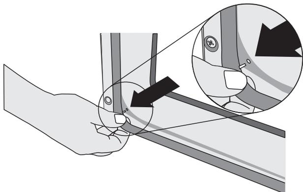
When fitting new seal, position the seal join at the bottom. Hook the new seal in one of the corner holes of the door, and proceed round the door snapping in each hook in turn.
