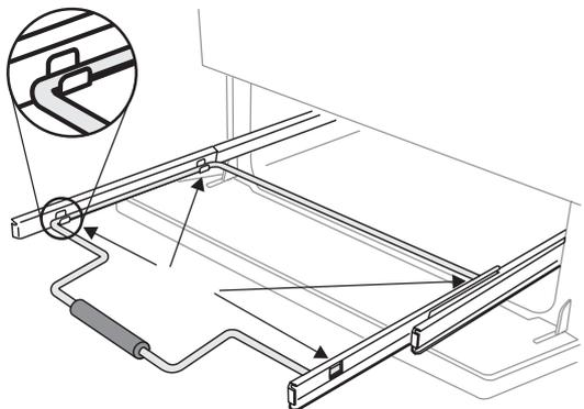
For each side, support the side rail with one hand and with the other hand lift the frame up and out of the side clips.
