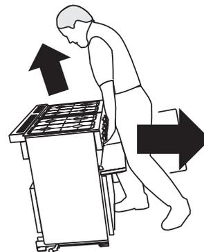
Lift the front of the cooker slightly and pull forward.
