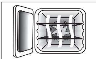
The left hand oven is a Multi-function oven. As well as the oven fan and fan element, it is fitted with two extra heating elements, one visible in the top of the oven and the second under the oven base. Take care to avoid touching the top element and element deflector when placing or removing items from the oven. For more detail on this oven see the section 'Multi-function oven'.
