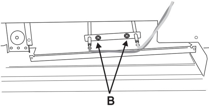
Remove the 2 screws B, holding the element to the bottom sheet.
