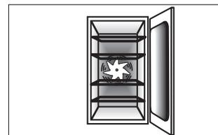
The fan in the right hand oven circulates hot air continuously, which means faster more even cooking. The recommended cooking temperatures for a fanned oven are generally lower than a non-fanned oven.
