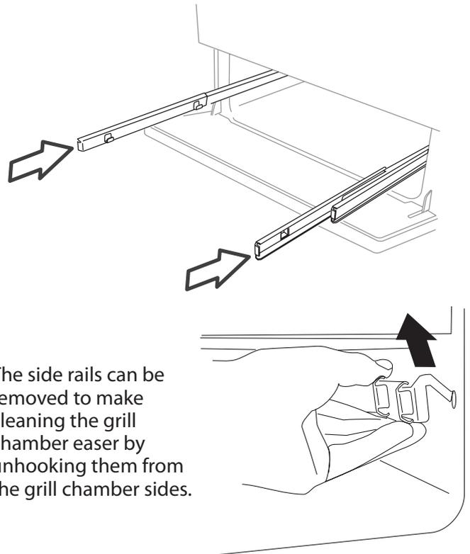
The side rails can be removed to make cleaning the grill chamber easier by unhooking them from the grill chamber sides.
