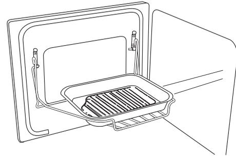
*The maximum weight than can be held by the Handyrack is 5.5kg (12lb). It should only be used with the supplied meat tin, which is designed to fit the Handyrack. Any other vessel could be unstable.*
