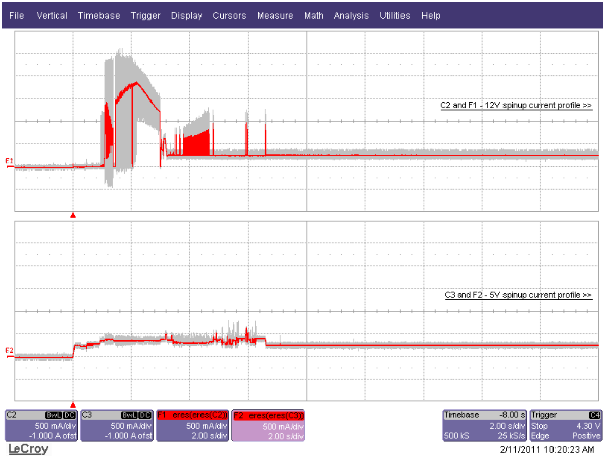
Figure 3. Typical 500GB model 5V & 12V startup and operation current profiles
