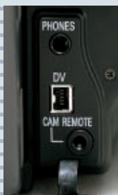
Terminals for headphone, digital interface, and camera remote. Split cover allows access to headphone terminal only.
