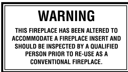
Figure 5 - Fireplace Warning Label
