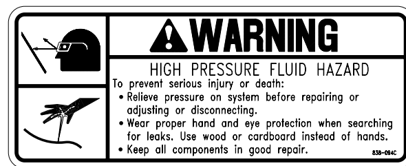
838-094C (Hydraulic Chute Option) Warning: Hydraulic Pressure
