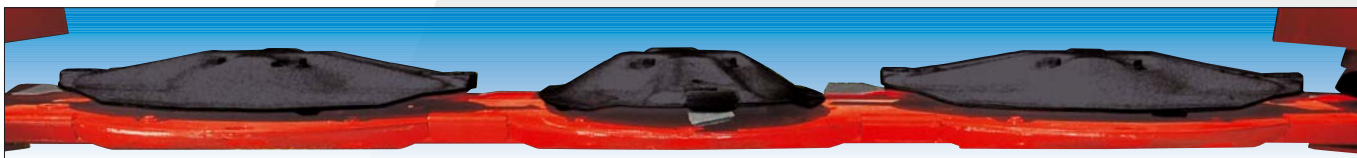
Very flat and smooth cutterbar that reduces soil or crop residues building up
