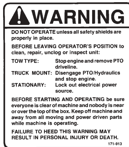
Figure D WARNING, DO NOT OPERATE UNLESS SHIELDS ARE IN PLACE Part Number 171-913 1 Required ALL MODELS
