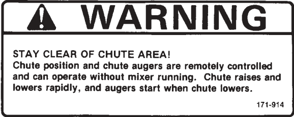
Figure E WARNING, STAY CLEAR OF CHUTE AREA Part Number 171-914 2 Required ALL MODELS
