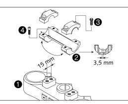
For this purpose, remove screws ③ of the handlebar clamps and screws ④ of the handlebar support. Position handlebar support, and tighten screws ④ to 40 Nm (30 ft.lb). Mount handlebar and handlebar clamps, and tighten screws ⑤ to 20 Nm (15 ft.lb). The gap between handlebar support and handlebar clamps is to be of equal size in the front and in the rear.
