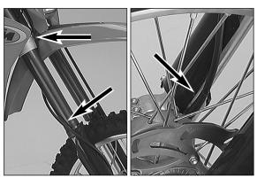
The speedometer shaft must be placed as running along the outside of the fork guard and pas the triple clamp toward the speedometer. Mount the collar nut **④**, turn the speedometer drive such that the speedometer shaft leads upward parallel to the fork log (see plots), tighten the
