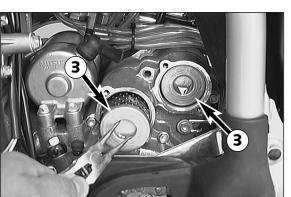
Using circlip pliers, you may now pull the oil-filter inserts  $\ensuremath{\mathfrak{G}}$  out of the housing.
