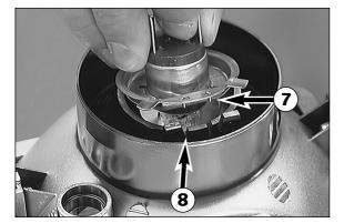
Insert new lamp such that the noses **⑦** engage the recesses **⑧** .When doing so, do not touch the glass body of the lamp so that it remains free from fat. Engage retaining clip, mount rubber cap and connector. If the parking-light lamp is to be replaced, simply insert it into the holder. Reinsert parking-light lamp together with holder.
