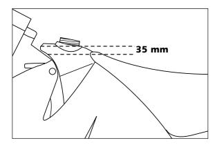
Fuel expands when its temperature rises. Therefore do not fill the tank to the top (see fig.).
