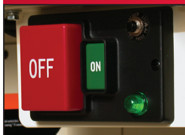
Moveable power switch with reset and power light
