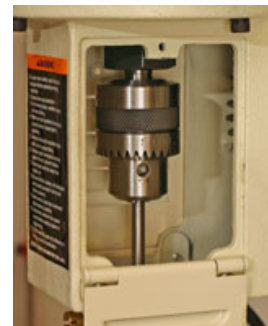
Swing down doors on both sides provide easy access to the chuck for working with the auger bits
