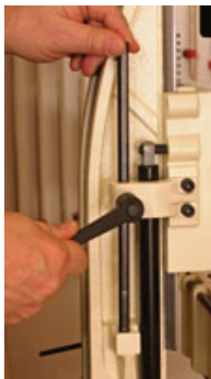
The tool-free depth stop is mounted close to the line of force so there is no deflection of the bit.
