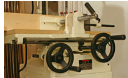
Large handwheels provide smooth, accurate control over the table movements.
