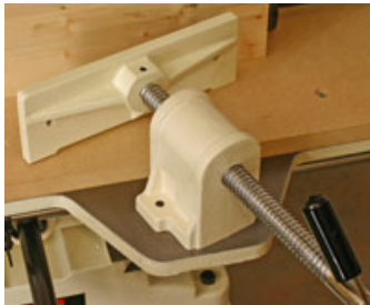
The large work vise has a special quick-adjust feature, plus it can be rotated to make clamping angled or odd shaped work pieces much easier.
