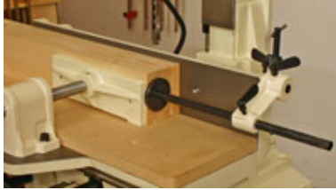
The large work table surface and the adjustable stop make cutting several mortises fast, easy and accurate.
