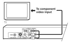
Use a component video cable (not supplied) to connect the COMPONENT VIDEO OUT jacks to a component video input on your TV, monitor or AV receiver.
