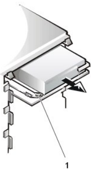
Figure 11. Diskette Drive Removal
