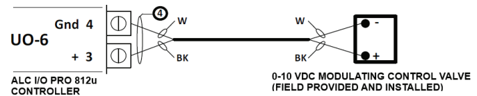
Fig. 12 — Hot Water Coil - Control Valve Wiring
