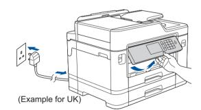
Connect the power cord. The machine will power on automatically.
