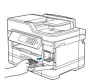
Open the ink cartridge cover, and then remove the orange protective part from the machine.
