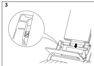
Load paper into the multi-purpose sheet feeder.
