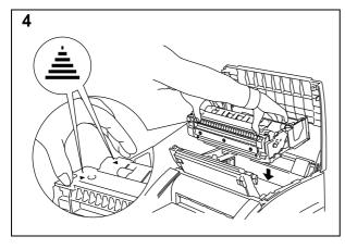
Install the drum unit into the printer.
