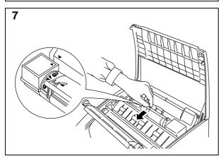
Gently pull the blue shutter lever on the toner cartridge forward until the red arrows are aligned.
