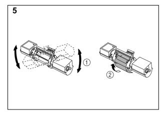
Unpack the toner cartridge and gently rock it from side to side well before installing. ( ① )
