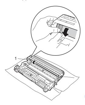
When you have found the mark on the drum that matches the print sample, wipe the surface of the OPC drum with a dry cotton swab until the dust or glue on the surface comes off.
