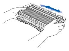
Put the drum unit assembly into the machine until it clicks into place.
