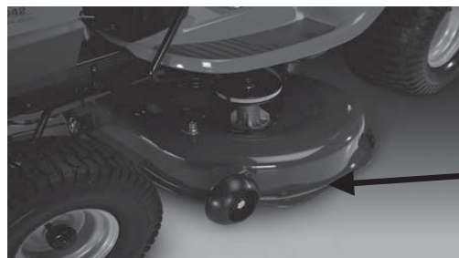
Stamped Deck Shell below, NOT reinforced
