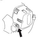
Choke: Set the choke control in the choke position.
