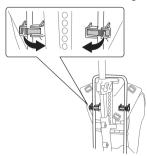
· Loosen the backplate from the frame on one side.
