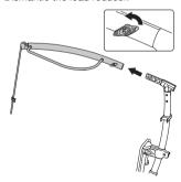
Position the load reducer as shown and fasten it.
