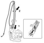
Dismantle the shaft. Loosen the coupling by turning the knob (at least 3 times).
