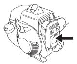
Some mufflers are equipped with a special spark arrestor screen. If your machine has this type of muffler, you should clean the screen at least once a week. This is best done with a wire brush.
