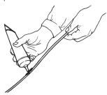
5 Slide the drive shaft back into the sleeve. Make sure the shaft engages correctly by turning it and pushing at the same time.
