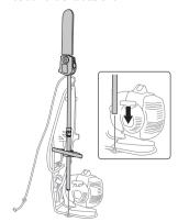
Wind the cord around the load reducer and the shaft, then fasten it as shown.
