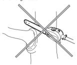
Use the stop at the base of the cutting head to provide support during cutting. This will help prevent the cutting attachment from "jumping" on the branch.
