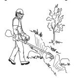
4 Switch off the engine before moving to another area. Fit the transport guard before carrying or transporting the equipment any distance. 5 Never put the machine down with the engine running unless you have it in clear sight.
