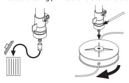
Screw the trimmer head onto the shaft.
