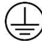
Figure 4. Equipment Earth (Ground) Point
