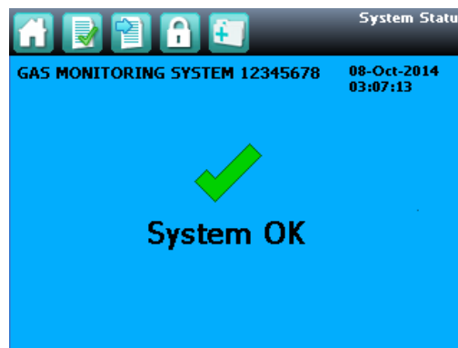
Figure 30. System Status Normal
