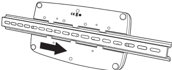
2. Then, using the appropriate hardware above, secure the DIN rail to the desktop.
