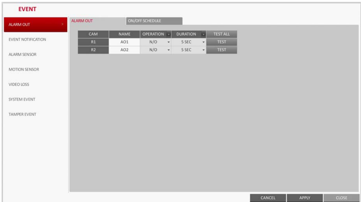
Figure 4-45 Alarm Out Screen
