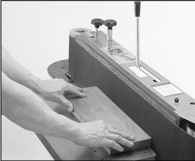
Figure 23. Edge sanding process.
