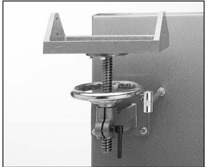
Figure 6. Installing the lead screw assembly.
