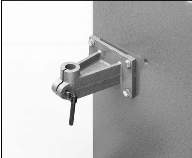
Figure 4. Lead screw bracket Installed.
