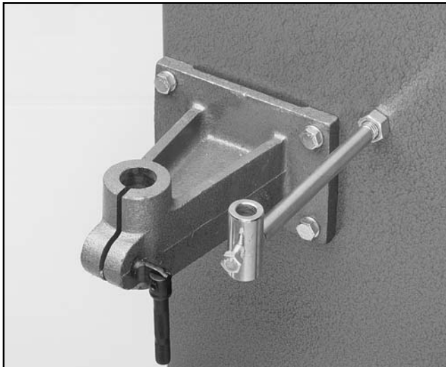
Figure 5. Installing the horizontal brace.
