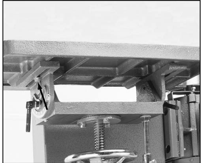
Figure 10. Attaching the working table.
