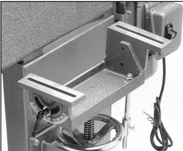
Figure 9. Table trunnions installed.
